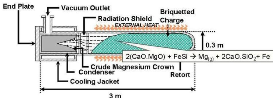
Figure 1. Pidgeon Reactor
