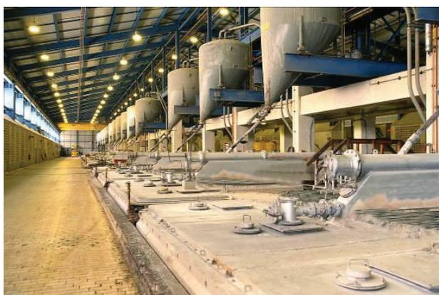
Figure 4. Norsk Hydro Magnesium Electrolysis cells at Becancour, QC
