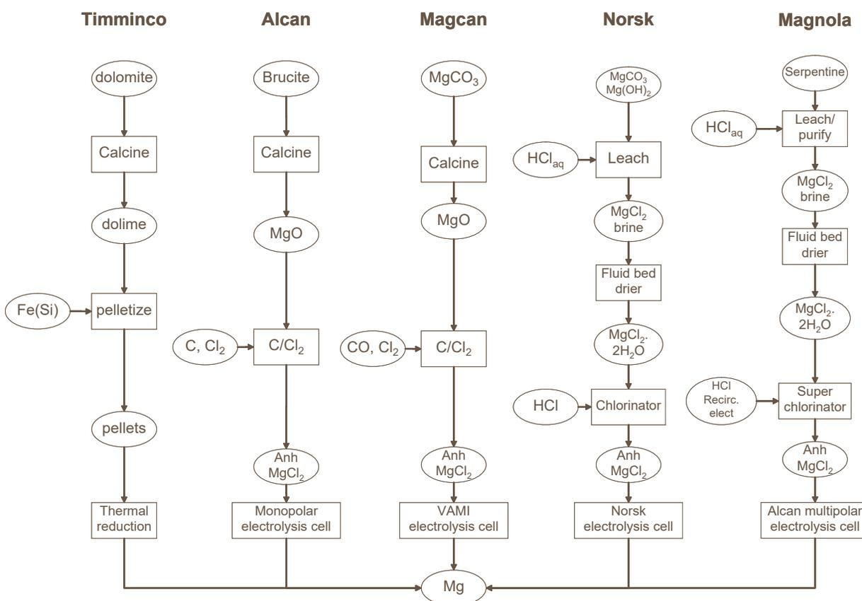
Figure 6. Side by side comparison of processes used in Canada
