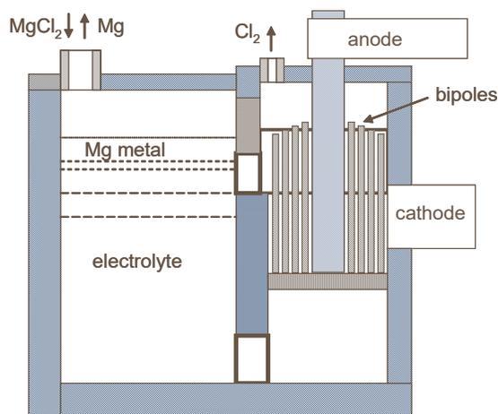
Figure 2. RTA Magnesium Multipolar Electrolysis Cell
