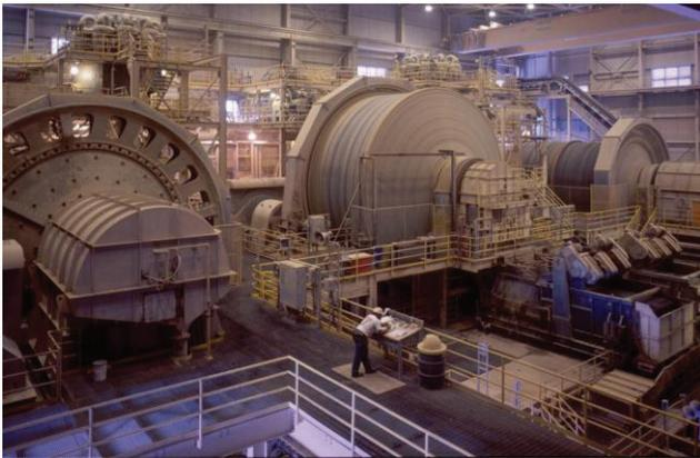
Figure 3. Ball mill and SAG mill in a cyanidation plant
