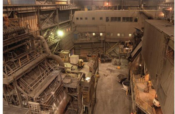
Figure 6. The Horne smelter with the Noranda Reactor on the left and the Noranda Converter on the right
