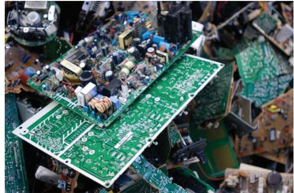
Figure 10. End-of-life electronics, an example of the more complex secondaries recycled today
