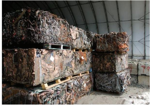
Figure 8. Bales of #2 copper, an example of a traditional type of copper scrap
